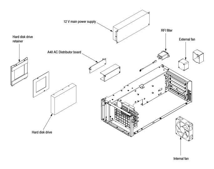
Figure 4-4: Internal modules
