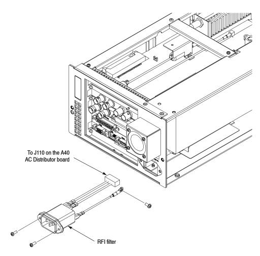
Figure 4-14: RFI filter removal
