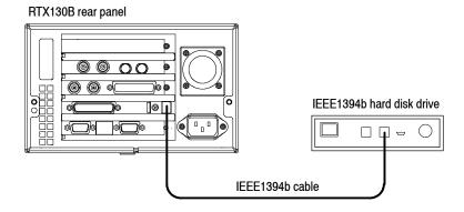
Figure 3-19: Equipment connection for checking the IEEE1394b interface
