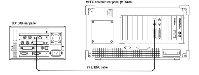
Figure 3-12: Equipment connection for checking the ASI record operation
