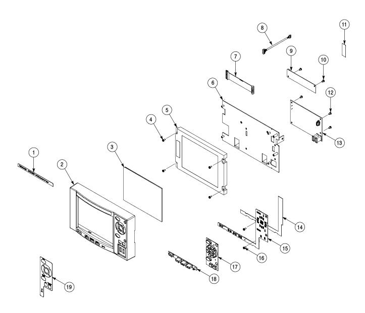
Figure 7-4: Front-panel unit
