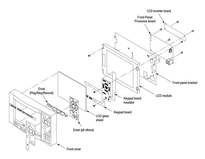
Figure 4-9: Disassembly of front-panel assembly
