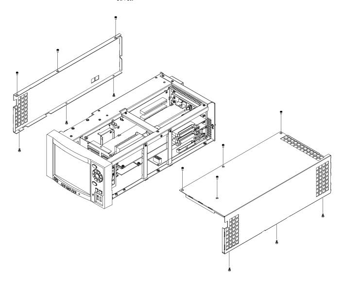
Figure 4-7: Right-side and left-side cover removal
