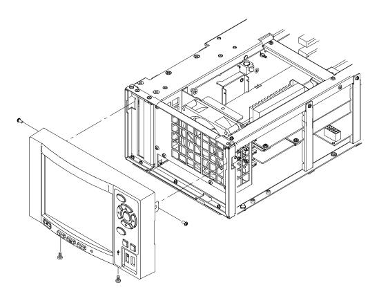
Figure 4-8: Front-panel unit removal
