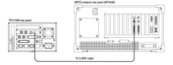
Figure 3-15: Equipment connection for verifying the 8VSB record operation
