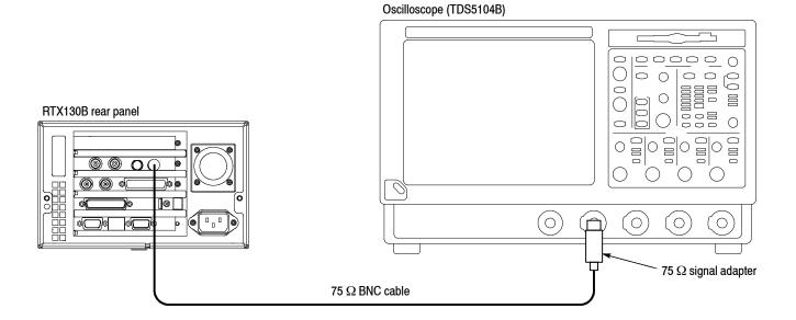
Figure 3-10: Equipment connection for checking the output signal-ASI interface
