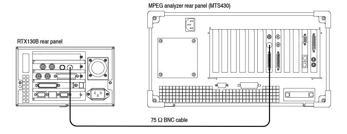
Figure 3-11: Equipment connections for checking the ASI play operation
