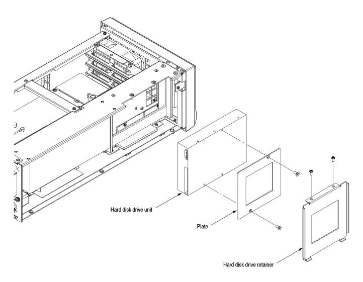
Figure 4-11: Hard disk drive removal
