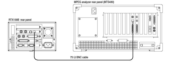
Figure 3-14: Equipment connection for verifying the 8VSB play operation
