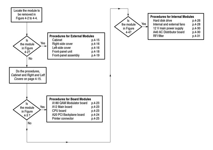
Figure 4-5: Guide to removal procedures
