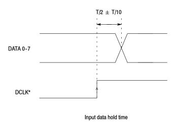
Figure 1-1: Timing diagram of the SPI interface
