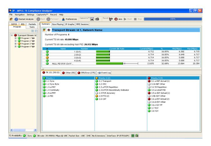
Figure 3-27: MTS400 Series TS Compliance Analyzer display
