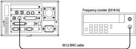
Figure 3-7: Equipment connection for checking the internal clock frequency
