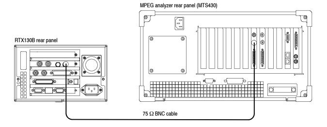
Figure 3-13: Equipment connection for checking the recorded file- ASI interface
