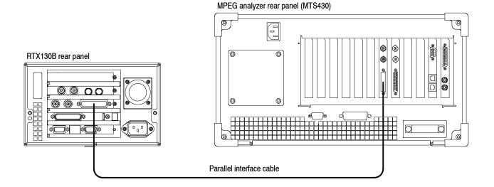
Figure 3-8: Equipment connection for checking the play operation-SPI interface
