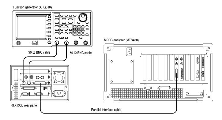
Figure 3-9: Equipment connections for checking the external clock/reference and trigger inputs
