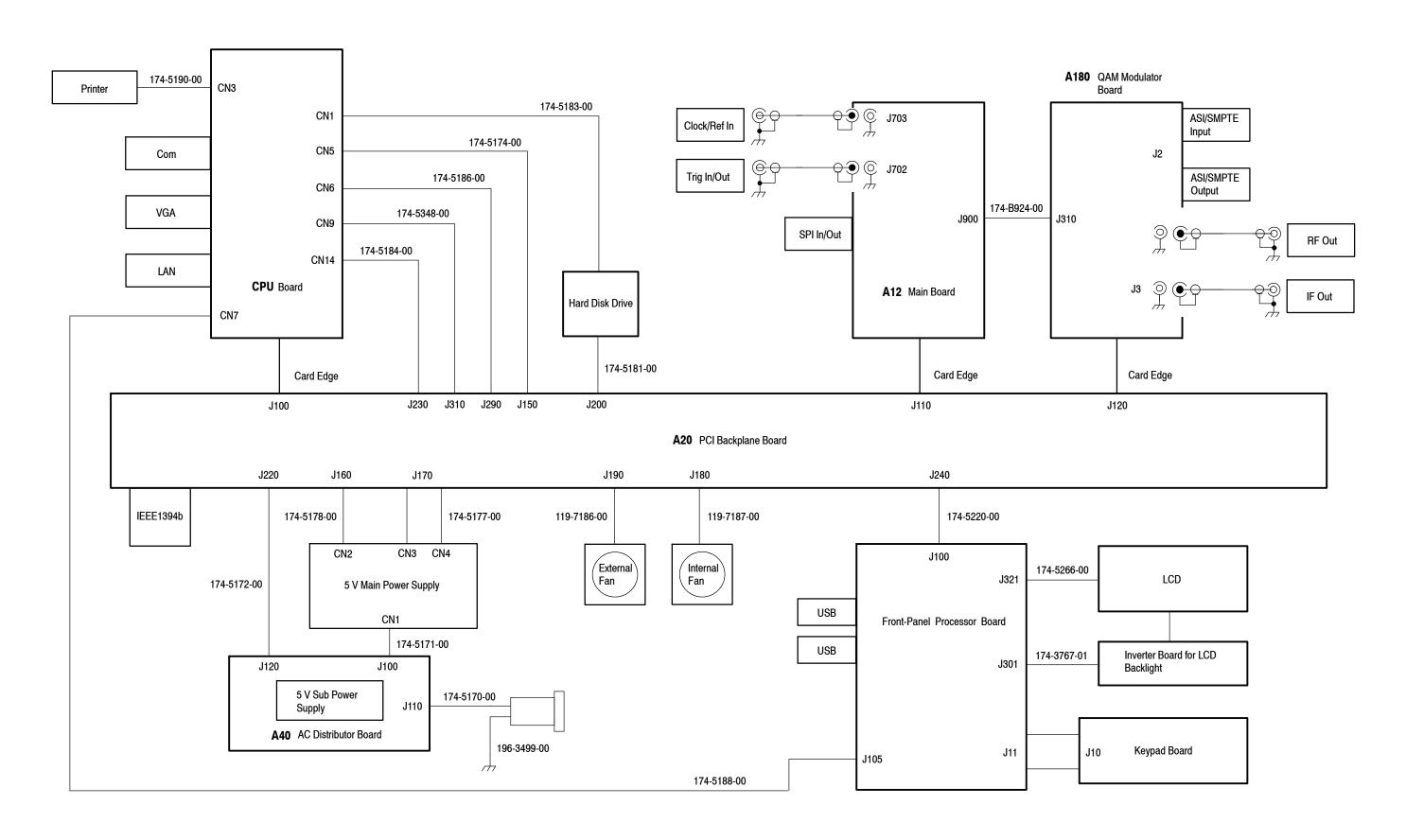
Figure 6-2: RTX130B interconnect diagram
