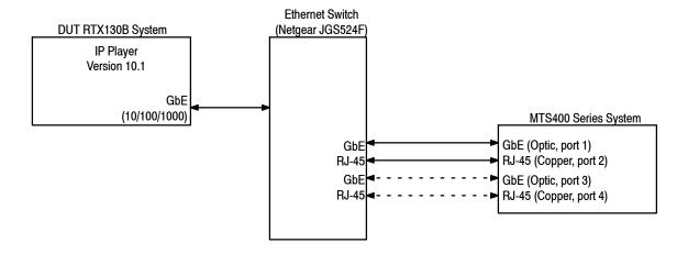
Figure 3-20: Equipment setup for Option GbE performance verification
