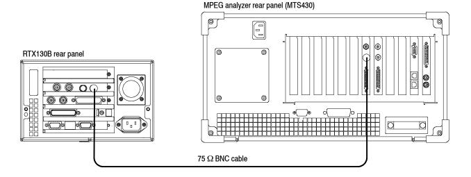
Figure 3-16: Equipment connection for verifying the recorded file-SMPTE310M interface
