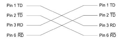
Figure 3-1: Pin connections for a crossover Ethernet cable
